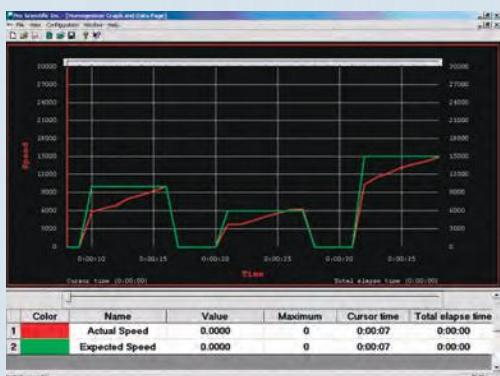
PROgrammable® Software graphs a homogenization program in real time on your computer screen
